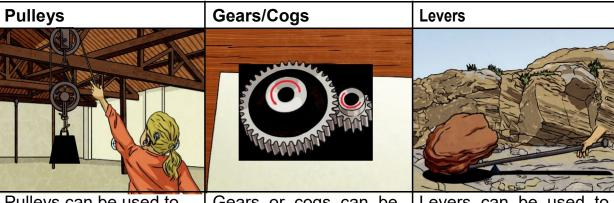
Pulleys can be used to make a small force lift a heavier load. The more wheels in a pulley, the less force is needed to lift a weight.
